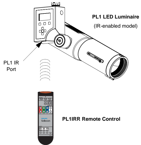
Figure 3: PL1 LED Luminaire Programming / Control
